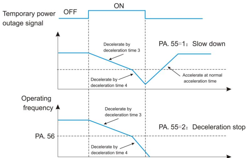
Figure 6-34 Level diagram of the FDT function
