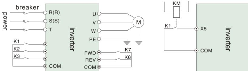
Figure 6-16 Multi-speed operation wiring diagram
