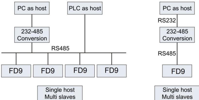
*Figure 9-1 Schematic diagram of the unit network*
