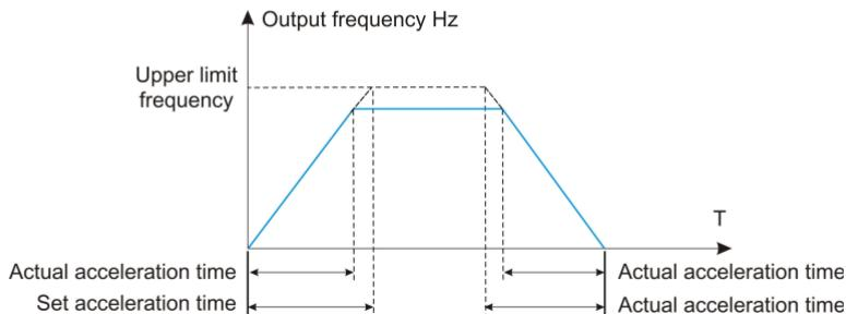
Fig. 6-1 Acceleration/Deceleration time
