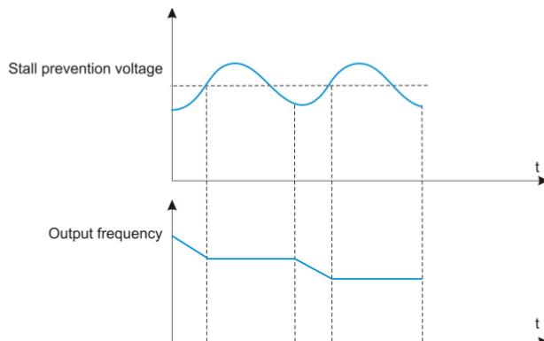
Figure 6-33 Over voltage stall function
