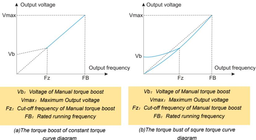
Fig.6-24 Manual torque boost
