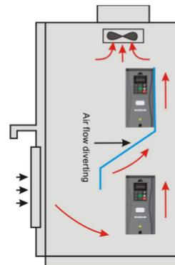
Figure 3-2 Mounting of multiple inverters
