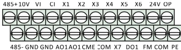
Fig. 3-6 Sequence diagram of control board terminal
