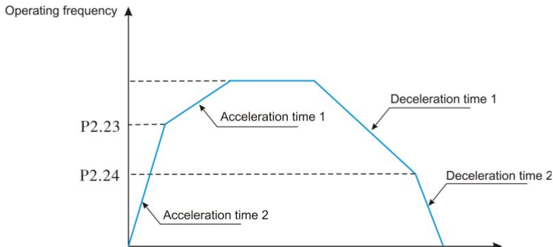
Fig. 6-12 Acceleration/deceleration switching
