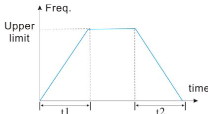
Fig. 6-03 Linear acceleration and deceleration
