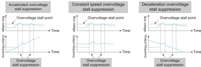
Figure 6-39 Schematic diagram of overvoltage stall action
