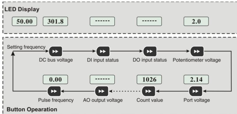
Fig.4-7 Example for running status data display operation
