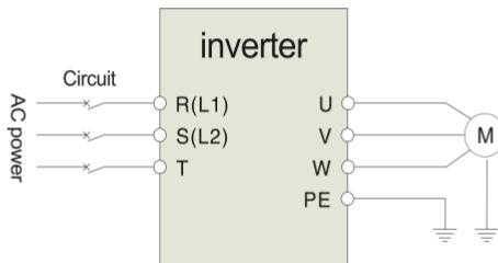
Fig. 3-3 Main circuit wiring
